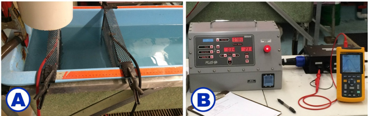
Figure 2. Electrified field exposure system consisting of a fiberglass exposure tank with iridium oxide-coated titanium mesh electrodes (A) and a Midwest Lake Electrofishing Systems Infinity Control Box ® with a connected resistor box (B) (Photographs by James A. Luoma).
