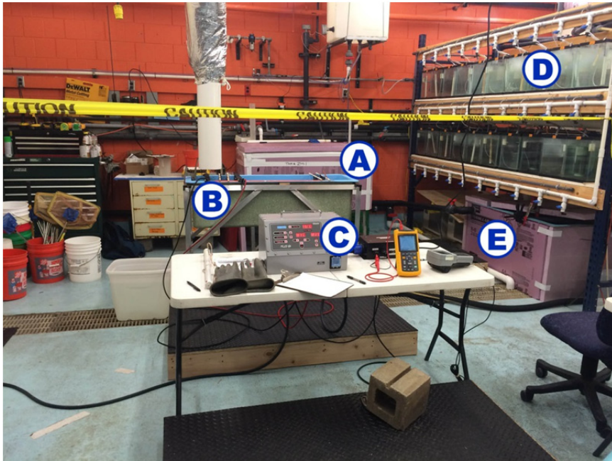
Figure 1. Combined temperature-controlled, semi-recirculating rearing, exposure, and post-exposure holding system, consisting of a 350-L zebra mussel rearing tank (A), an exposure tank (B), an electrofishing control box (C), a post-exposure holding system (D), and a recirculation sump (E) (Photograph by James A. Luoma).
