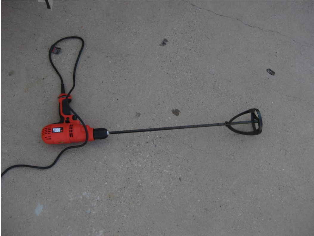
Fig. 3 Drill mounted paint mixer
